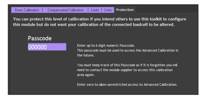
You can protect the module against a standard user being able to enter any of the Advanced Calibration pages of the DSC Toolkit.
