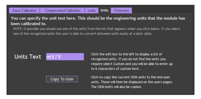
If you have calibrated the module to standard units you can specify them here. The advantages are that the standard user will see the units displayed and if the units are recognised by the software the standard user can simply convert to another unit scale without recalibration.
