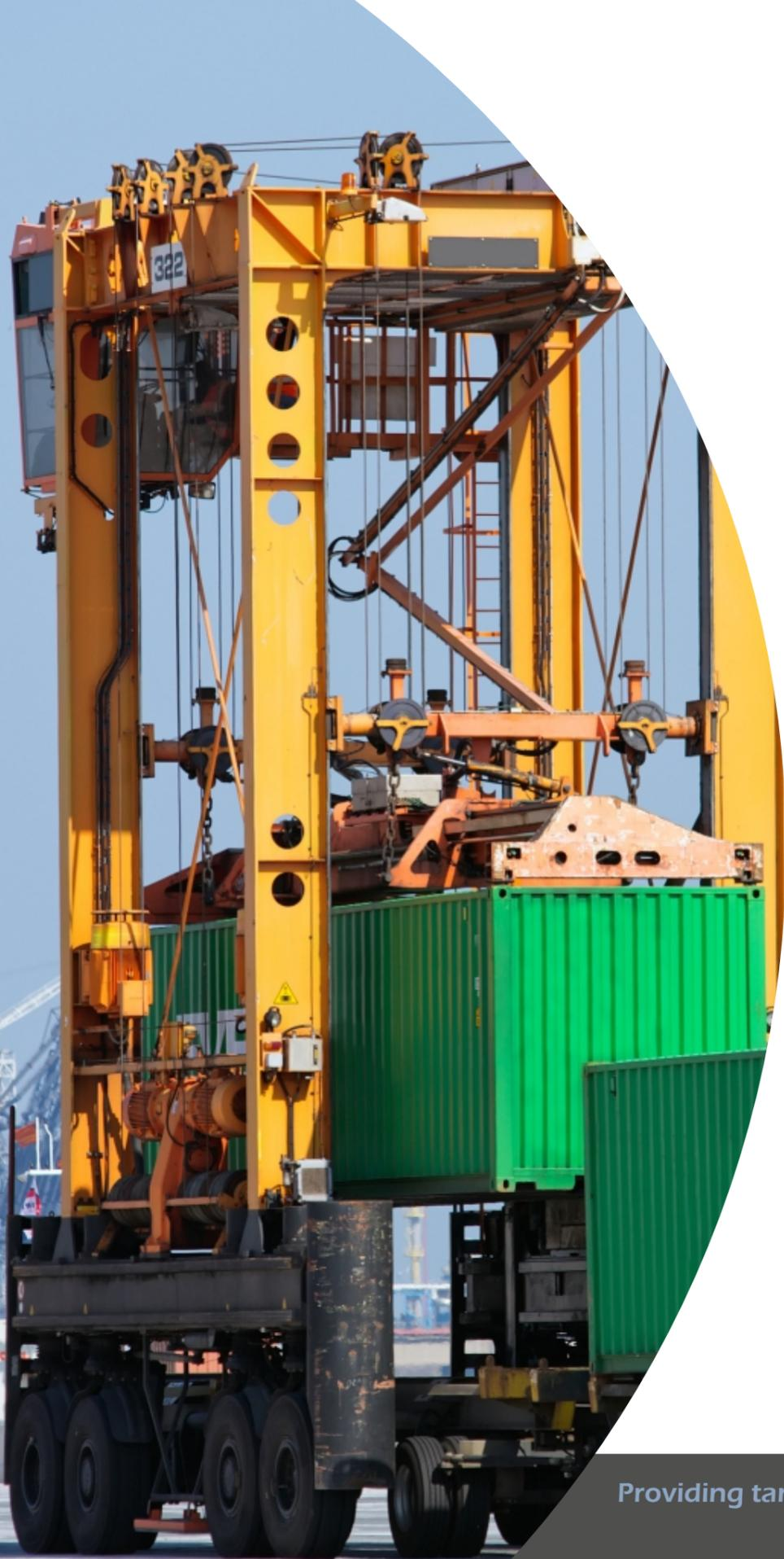
The LCM Systems container weighing system has been designed to be easily retrofitted into the spreader or headerblock of straddle carriers, container cranes and telehandlers. It can be tailored to meet the needs of the individual port, with the standard package being a stand alone system, but with options for a system that is fully integrated into existing terminal operating systems (TOS).
