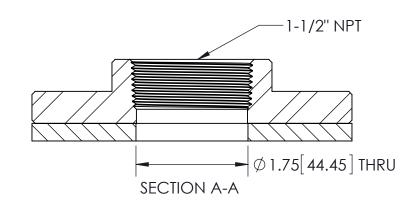
Flowline Part Numbers LM53-4855 = adhesive tank top fitting, 1 1/2" NPT, PVC
