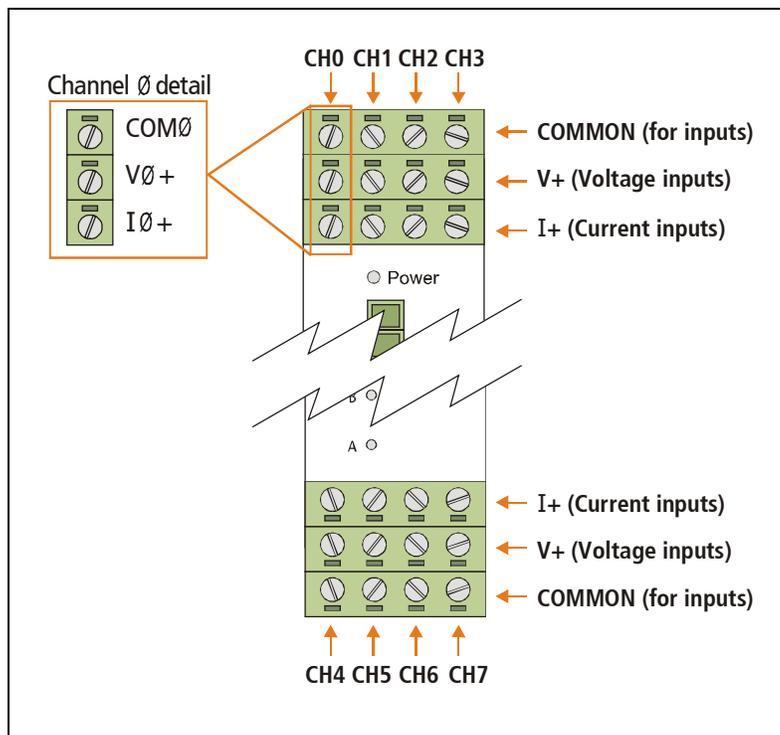
Figure 11 – Disposition of the analog inputs
