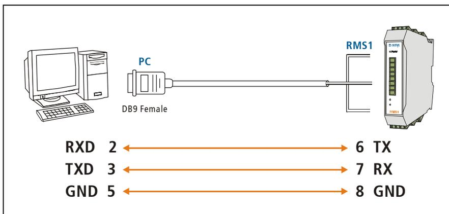
Figure 8 - RS232 connection to a PC
