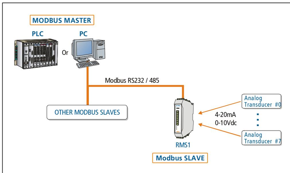
Figure 1 - Example of application for Modbus Slave
