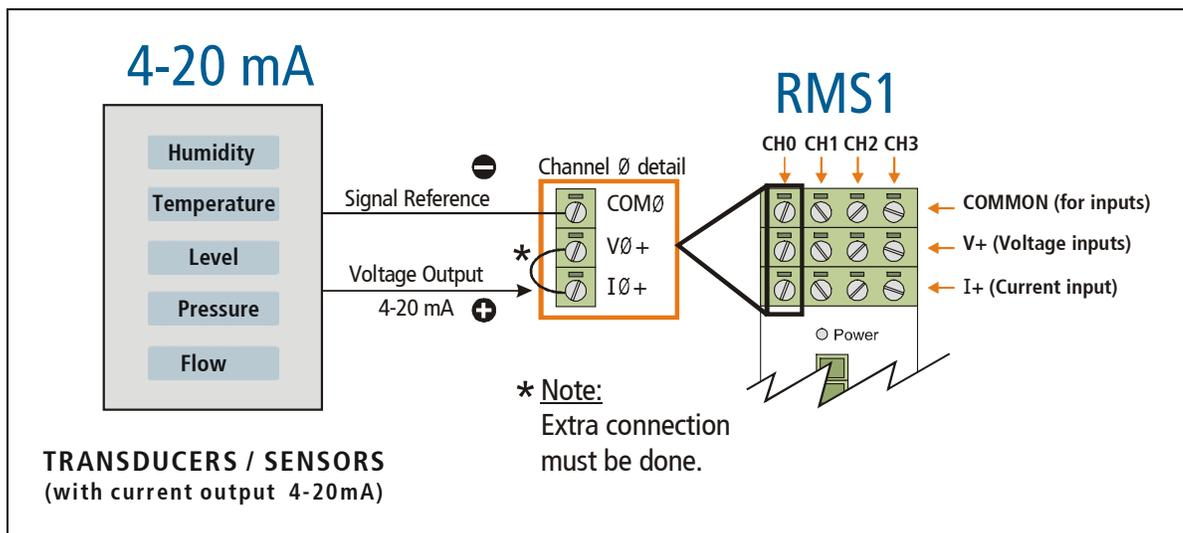
Figure 13 – Current loop sensors connection.
