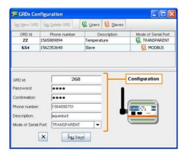
The Telephone and Description options are optional and not necessary. When we finish loading all necessary data we press the "Save" button to add the GRD/cLAN to the list.
