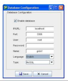
From here we can modify the configuration of the base, the IP address, the port, name and type of database (MySQL and SQL) containing the information and also configure the user and password so the MW can have access to the database.
