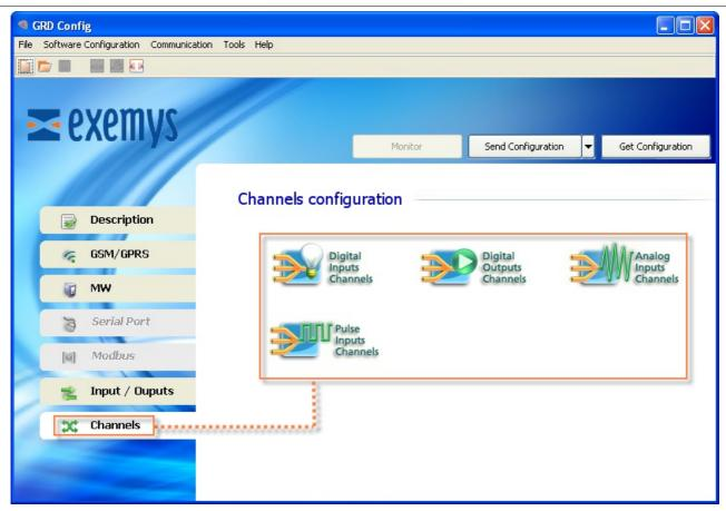
After selecting the desired channel and among any of the 4 you'll have the option to add or remove, it is important to point out that within each channel only inputs and outputs compatible with that channel will appear.
