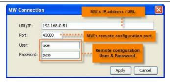
The IP to be loaded is the one the MW is running on, and the port is the one configured to have access to it.
