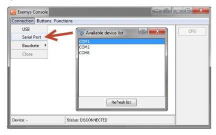
Power the device, and press the CFG button until you see a welcome message. You must do it within the first 7 seconds after powering the device on.
