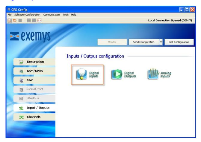
When we enter the configuration of a digital input we will see that we can configure 2 parameters one is the anti-rebound to avoid noise and the counting splitter in case of use as pulse input.
