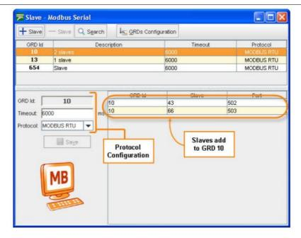
In this manner, the two GRDs are configured from the MW side and working according to what was established in the beginning.
