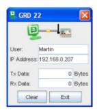
When the cLAN/GRD is connected and a user is connected to the MW pointing to that device, the screen will be shown as enabled.
