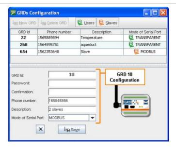
When you press the save button it is stored in the list of valid GRDs. The mode must be MB for it to work in this manner. The following figure shows the addition of the other GRD and in the upper part the GRD added previously.
