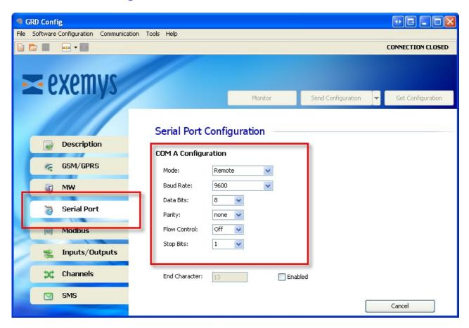
In GRD with two serial ports you will be able to configure them individually. **Notice that the two serial ports cannot be configured on the same mode**.
