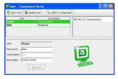
The configured user name and password are used for authentication of the port redirector. When a redirector connects to the MW it must indicate the user name and password.
