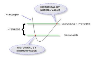
It is not possible to configure a value of hysteresis greater than the difference between the maximum and minimum, and also a maximum smaller than a minimum. We can also associate a digital output channel to the alarm event by maximum and another one of alarm by minimum, this means that when the analog input in the maximum range will activate an output and in the minimum another one.
