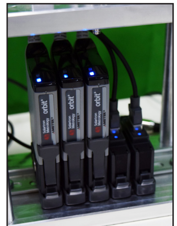
TCon4 provides compatibility with predecessor modules for all new and existing Solartron Metrology products
