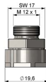
TM-TAS-CT Pivoted joint for CT sensors
