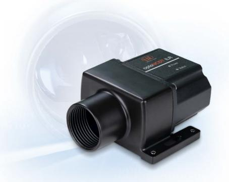
With the optoNCDT ILR3800-100, Micro-Epsilon presents a new powerful laser distance sensor. The sensor is designed for operation with or without reflector film, which is used depending on the distance and ambient conditions. The sensor measures large distances up to 100 m without contact and provides best results even on challenging (dark, structured or weakly reflecting) surfaces. The measuring range can be extended up to 150 m by attaching a reflector film to the measuring object.
