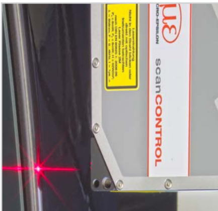
Gap measurement on a car body
