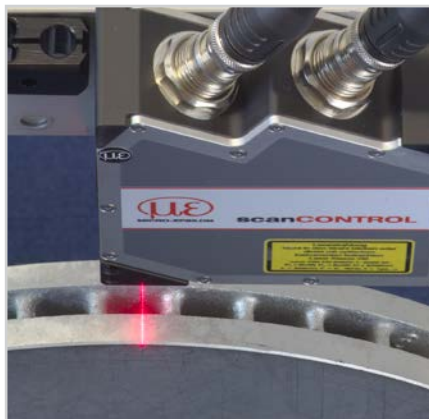
Profile measurements on brake disks
