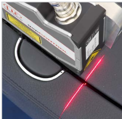
Distance measurement at the centre console
