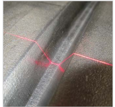
V-gap measurement on pipes
