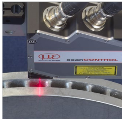
Profile measurement of the brake disc
