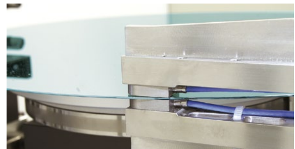
Wafer thickness measurement with two capacitive sensors
