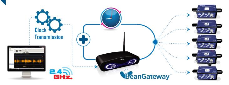
TimeSync function brings time-synchronization over the Wireless IIOT Sensors (±2.5ms of accuracy between each Wireless IIOT Sensors) and contributes to enhance user experience about correlation of remote sensing data and modal analysis
