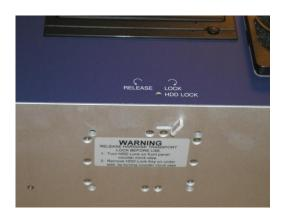
**IMPORTANT:** always lock the Hard Drive before shipping the PCM4. Failing to lock the Hard Drive will void warranty!
