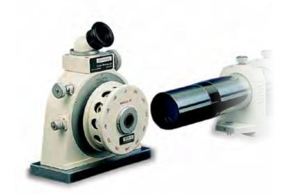
...checking the TB100 clinometer with the TA51 autocollimator
