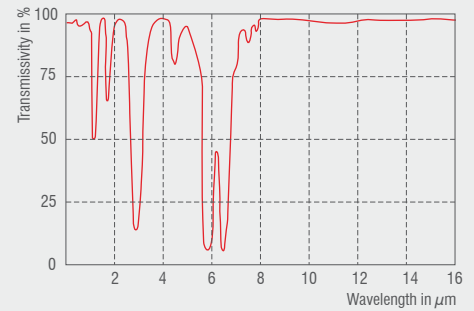
Spectral transmissivity of air (1m, 32°C, 75% r. f.)
