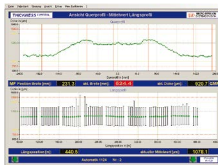
Combination profile8301.CT; vertical cursors show the points which are used for calender control
