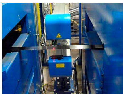
Thickness measurement in a grinding line
