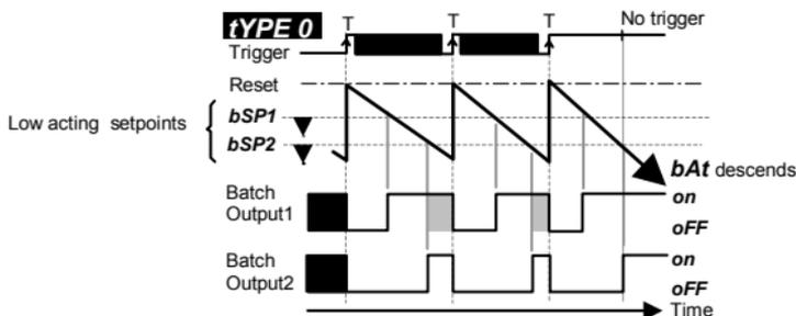
When **dir** is set to **uP**, the relay/TTL outputs are changed by the batch total rising above **high acting** setpoints **bSP-1** and **bSP-2**. When **dir** is set to **doWn**, the relay/TTL outputs are changed by the batch total descending below **low acting** setpoints **bSP-1** and **bSP-2**.
