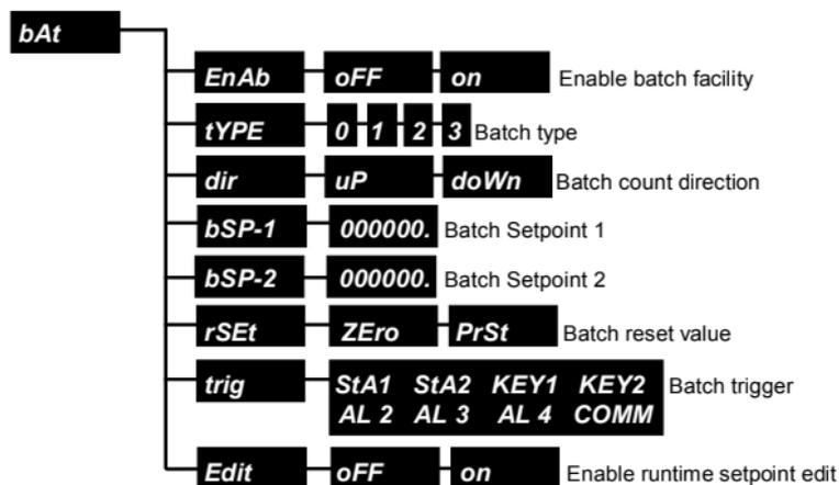
The batch control function uses the total **Ltot** from the totaliser to deliver successive batch totals **bAt** over time. The totaliser must be setup and enabled because the batch process uses the totaliser output **Ltot** as an input.
