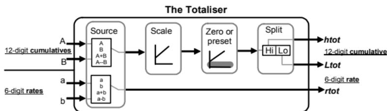
The values input to the totaliser depend on the mode of operation (*inPt*, *tyPE* setting). The **Accumulated** columns in the following table show which values are always fed to the totaliser for each particular operation mode.
