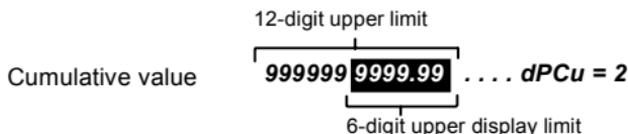
The totaliser can accept the whole 12 digits of a cumulative value and display it in 2 halves.
