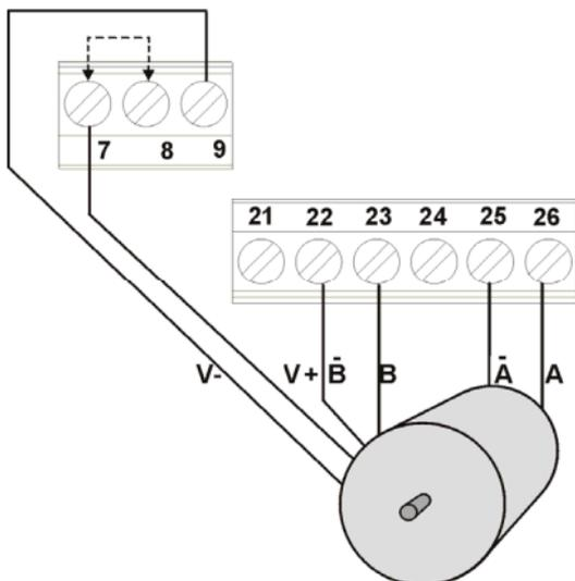
Note: Encoders are available with a range of output voltages and output types, for example, NPN (open collector) transistor, TTL and so on. Refer to the previous connection diagrams for wiring details.
