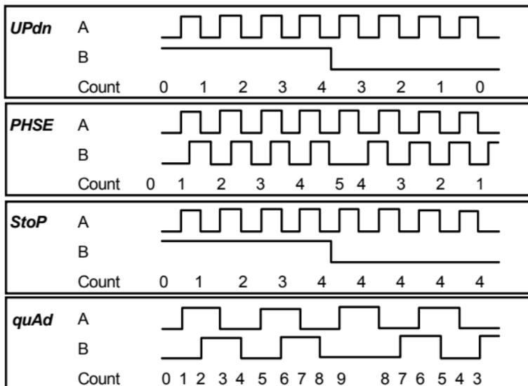
When the control style is ***uPdn*** and ***inVb*** is ***oFF***, the counter counts up when Input B is high (Input B voltage higher than  $V_B$ ) and counts down when Input B is low.
