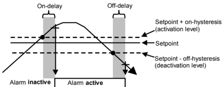
The effect of hysteresis on a high alarm is to raise the activation level by the on-hysteresis amount and lower the deactivation level by the off-hysteresis.
