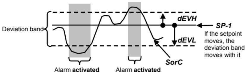
**dEVH** and **dEVL** appear in the Alarms menu only if the alarm type is setup as **dEV** for a deviation alarm. A deviation alarm is activated when the real time **SorC** value falls outside the deviation band.
