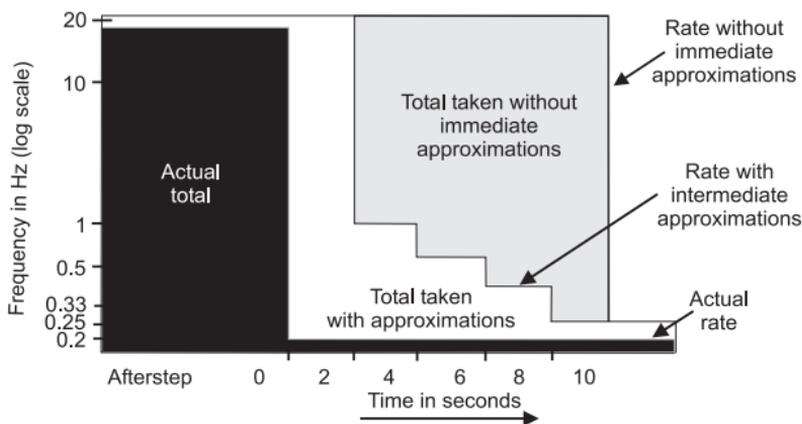
For example, if frequency is being measured and it is changed suddenly from **20Hz** to **0.22Hz**, over time, the instrument may display **20**, **1**, **0.5**, **0.33**, **0.25**, **0.22**. This is better than displaying **20** all the time until **0.22** is measured.
