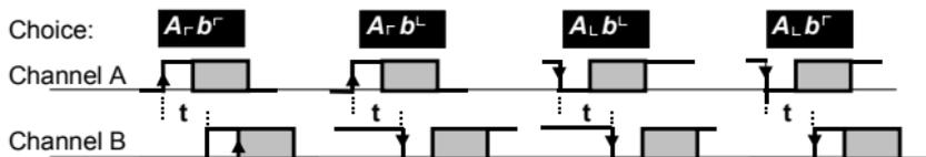
It does not matter if the Channel A pulse ends before or after the Channel B pulse begins or ends, but Channel B must be as shown when the sought edge on Channel A occurs or the display will not be updated. The sought edge is marked with an arrow on Channel A.
