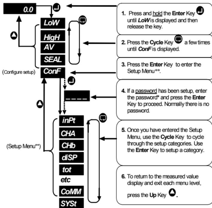
\* To enter the password, use the **Up/Down** Keys to edit the digit value and the **Cycle Key** to go to the next digit.
