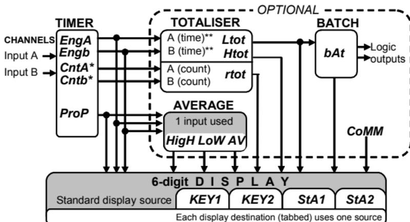
\* Period only. The measurement may be : period, pulse high time, pulse low time, duty high % or duty low %.
