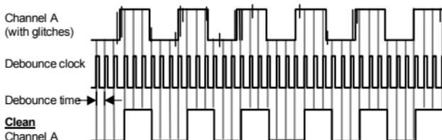
On each rising edge of the debounce clock, the instrument copies and latches the state of Channel A (and B) producing a Clean Channel A (and B). The resulting number of pulses is the same as the number input, but without the glitches caused by contact bounce. Without debounce, the glitches would also be counted.
