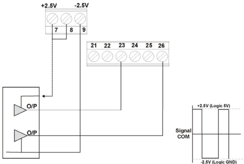
For PLC or other logic (TTL) output devices, the Transducer supply is configured to provide 5V (+/- 2.5V with respect to logic device signal common (GND /0V)). If the logic device provides its own supply then omit the connection to pin 7 of the instrument.
