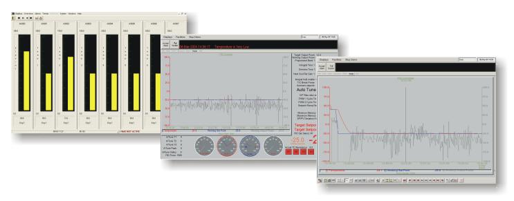
The Tracker 300 Series uses the widely available Modbus RTU protocol so is compatible with a huge range of data acquisition software packages, SCADA systems, HMI devices and web-enabled remote access packages. Data Track can provide software and HMI devices to suit most applications. Consult Data Track or your distributor for application advice.
